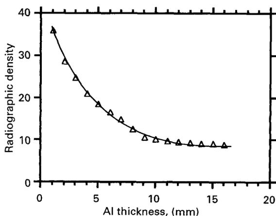
Figure 1 The calibration curve for the radiographic density of the aluminum step-wedge.
