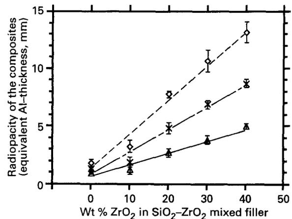
Figure 2 The effects of the ZrO<sub>2</sub> content in the fillers on the radiopacity of five experimental composite resins containing admixed SiO<sub>2</sub>-ZrO<sub>2</sub> fillers:  $\Delta$  1 mm;  $\times$  2 mm;  $\diamond$  3 mm.
