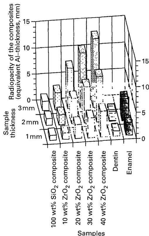
Figure 3 Three-dimensional comparison of the radiopacity of five experimental composite resins containing admixed SiO<sub>2</sub>-ZrO<sub>2</sub> fillers, human dentin and human enamel.
